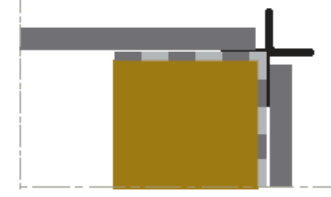
Figure 6: External Corner with trim Timber subframe
